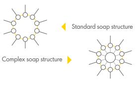
The thickener holds the oil and releases it under pressure or load to build up a protective lubrication layer keeping the metal surfaces in the application apart, e.g. between the housing and the rolling element in a bearing. This reduces friction and minimizes abrasive wear. When the pressure is released, the oil is re-absorbed into the thickener fibre matrix. You can think of this as acting in the same way as a sponge when pressure is applied and then released.
