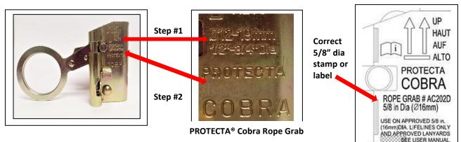
If the information in Step 1 and Step 2 is stamped onto the side of the rope grab as illustrated above, remove the unit from service immediately. <u>Owners of AC202D Cobra Rope Grabs can choose one of the following options for each affected rope grab they own</u>:
