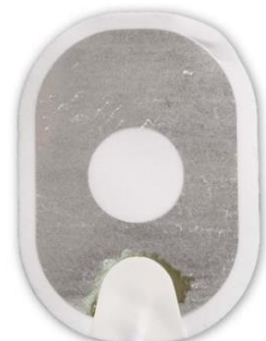
Figure 3: Gel almost completely separated from backing.
