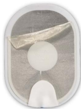
Figure 1: Separated gel that has folded onto itself when peeled.
