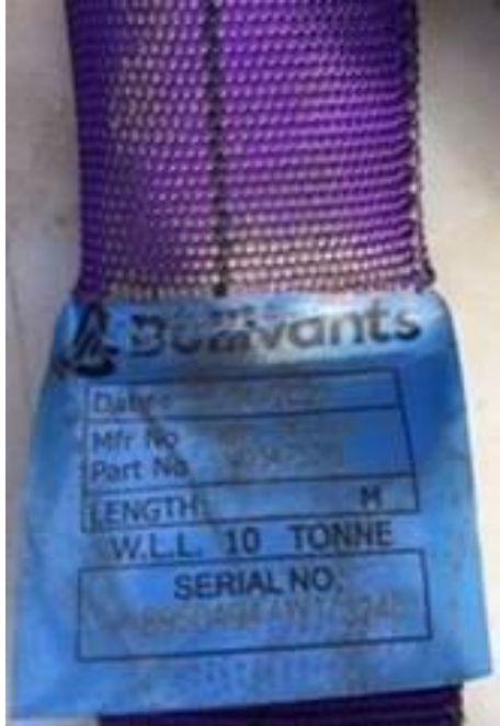
← Incorrect reference on label of 1 tonne sling to WLL of 10 tonnes
